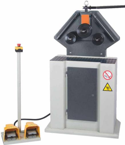
The PBM-30 Profile bender has 30 mm shafts and 2 driven bottom rolls driven either by a 1-Phase or a 3-Phase motor and comes with a standard set of section rolls that are configurable and are suitable for most bending applications of square or angular profiles. If you wish to bend round tubes or pipe, we have tools ready to go off the shelf for all common sizes such as 42.2 mm and 48.3 mm outside diameters along with many other sizes being readily available. If you are wanting to bend custom
