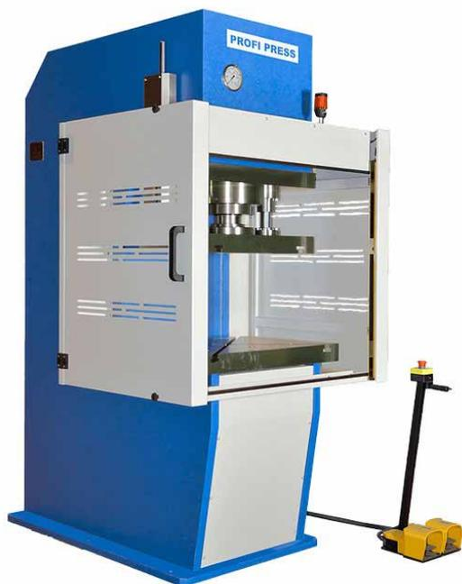
This 150-ton C-frame by RHTC Profi Press is suitable for performing work involving deep-drawing, forming and stamping, riveting, and many other applications. It has a throat depth of 375 mm and a working speed of 4 mm/s which is precluded by and an approach speed of 20 mm/s. After the cycle is completed the top plate returns at a rate of 31 mm/s. Maximum stroke of the top plate is 250 mm with the press having an overall shut height of 400 mm.
